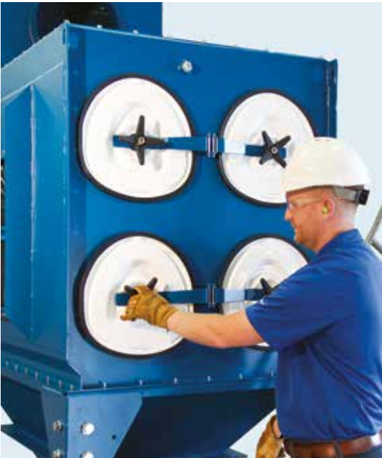
Loosen cover with 4-lobe knob. Knob has center lug enabling power tool operation.
